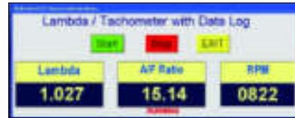
Here is a capture of the screen that shows and logs AFR versus Lambda versus RPM in real time.
