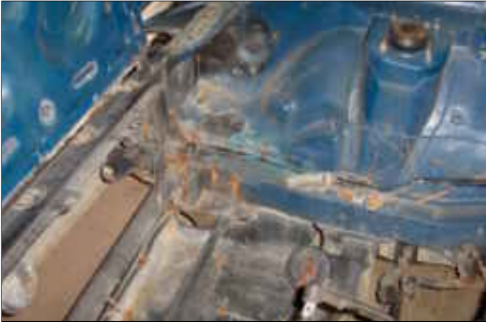
Passenger-side engine bay rust and wrinkles.
